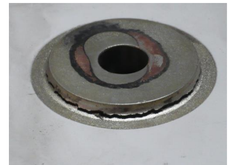
Cracked connection, test for Capacitor being charged
