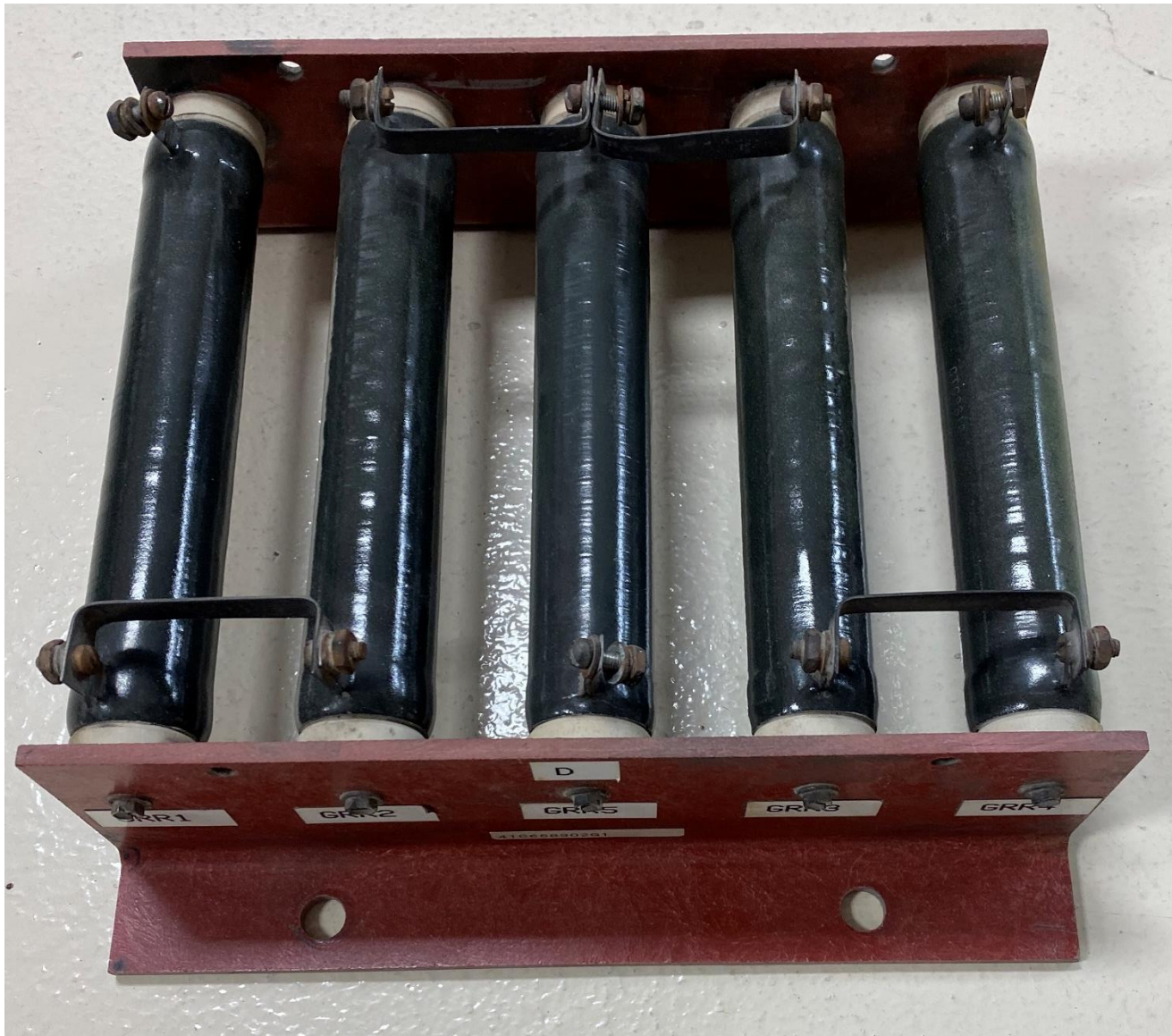
17FM402A1 GROUND REFERENCE RESISTOR PANEL
